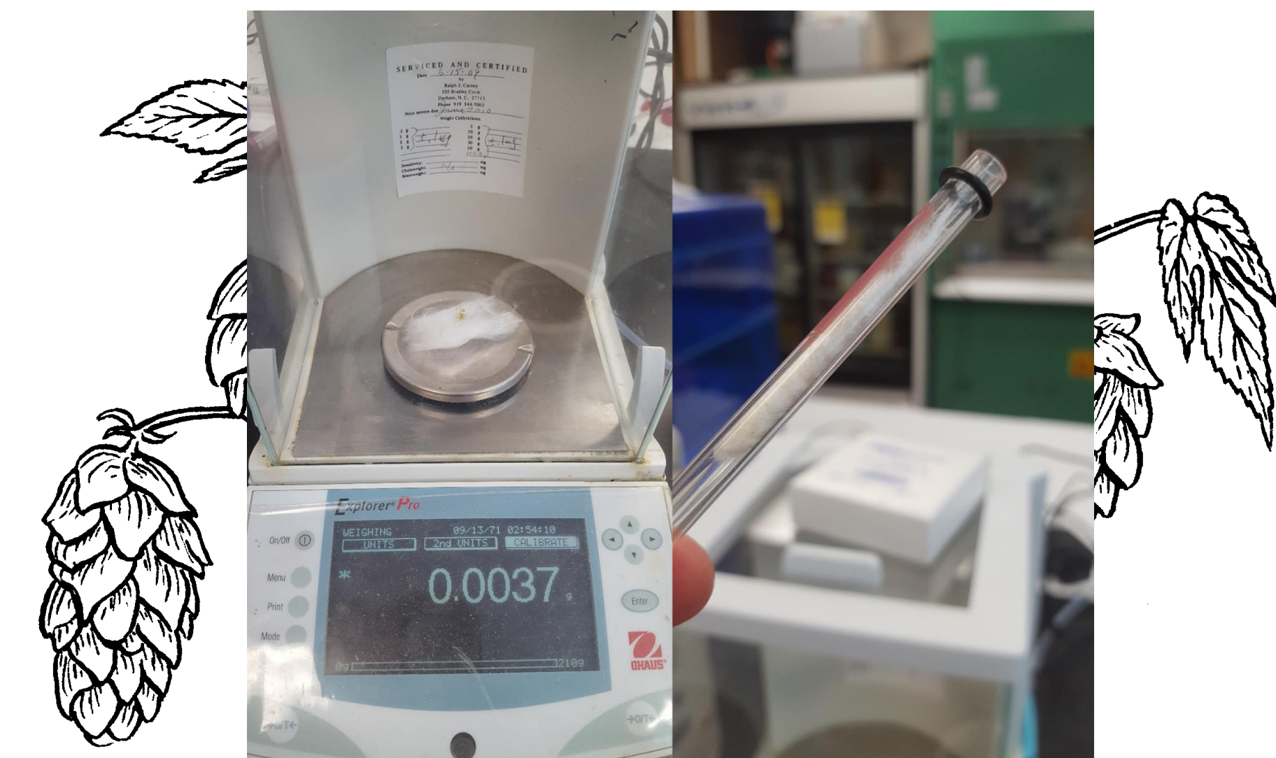
Figure 1. Example of a typical sample preparation. Simcoe hop pellet (3.7 mg) was weighed on tared glass wool by analytical scale (left). The resulting wool and pellet material were inserted directly into a clean GC liner (right), which was subsequently inserted into the GC-FID inlet.
